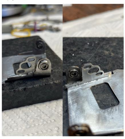
Example of Westrock BLMNZ mount fitted to C30 chassis. Shows how much of the original JK motor mount has been left intact to act as a lip to solder the bracket firmly against, and second shot shows how the rear leg of the Westrock mount extends over the flat surface of the C30 to just behind the pillow block.
