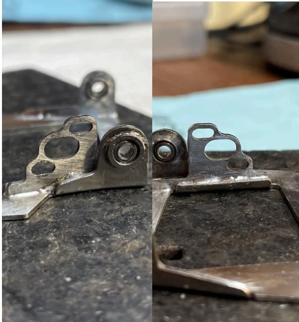
Example of the Westrock bracket mounted flush (ie against and parallel) with the existing motor mounting lip – it is hard up against the motor mounting lip, it sits in the “groove” between the motor mounting lip and the foot of the pillow block, and it benefits from some bracing from solder between the mount and the foot of the pillow block.
